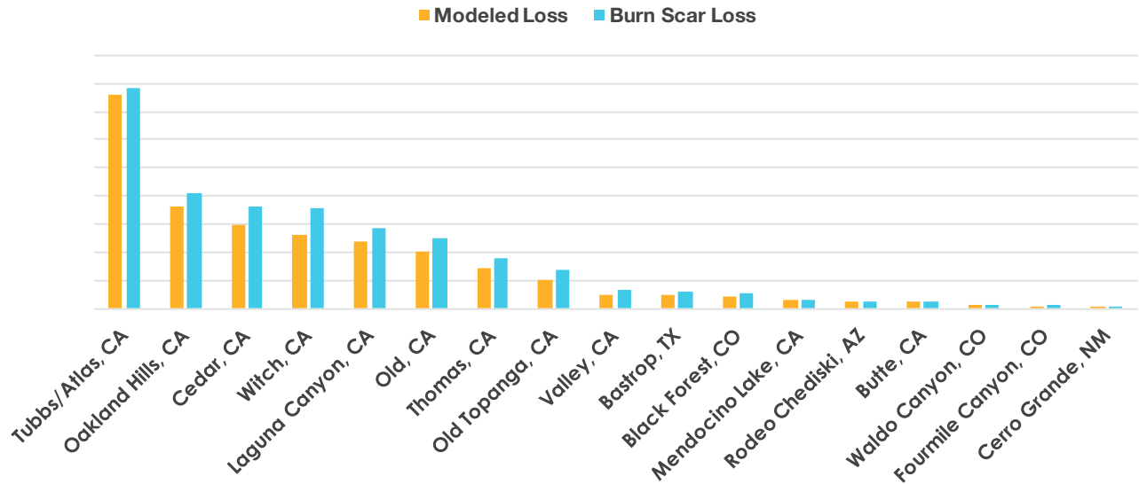
Modeled and burn scar losses for the 17 significant historical events included in the AIR Wildfire Model for the United States show good agreement.
